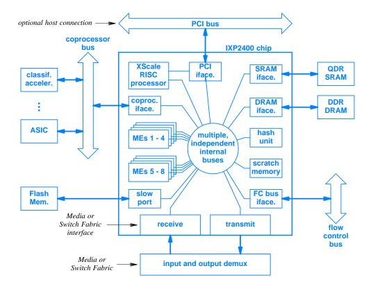
**Figure 15.10** Illustration of the internal architecture of Intel's IXP2400 network processor. The eight microengines and the RISC processor are programmable.
