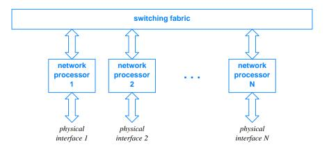
**Figure 15.12** Conceptual organization of a packet processing system that uses Motorola's C-Port network processors. Each network processor can handle both ingress and egress.
