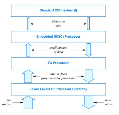
**Figure 13.7** Illustration of packet flow through the processor hierarchy. Performance is maximized when lower levels handle packets locally without passing them up the hierarchy.
