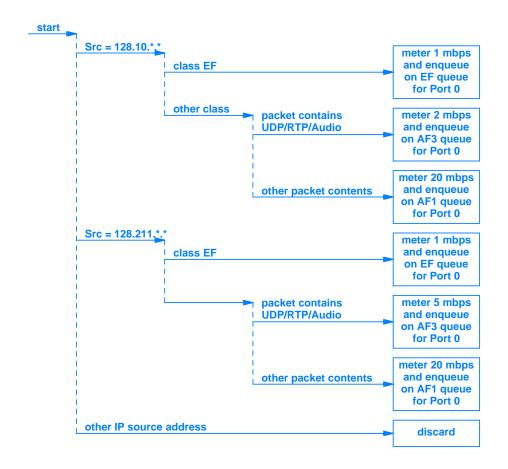
**Figure 24.8** The decision tree for packets that arrive on Port 2. The IP source address in a packet is used to select an appropriate action.
