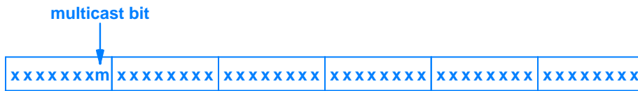
Figure 3.4 The multicast bit in a 48-bit Ethernet address is the low-order bit of the high-order octet. Unicast addresses have the bit set to 0, and multicast addresses have the bit set to 1.
