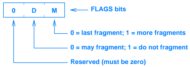
Figure 5.3 Bits in the FLAGS field of an IP datagram and their use in fragmentation. Most datagrams start with the three bits all set to zero.
