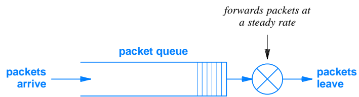
Figure 6.1 Illustration of a leaky bucket traffic shaper. As they arrive in bursts, packets are deposited in a queue. The leaky bucket mechanism then forwards one packet at a time. The analogy with a water bucket is appropriate.
